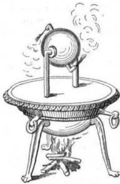
Heron's æolipil Roterende dampkugle
